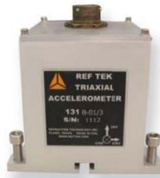
The 131B-01/3 model is a  $\pm 4g$  full scale accelerometer with  $2\mu g^2/Hz$  noise level and is best suited for structural applications (building, bridge, dam monitoring) when the project requires accelerometers in triaxial configuration.
