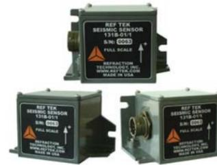
The 131B-01/1 shown here is  $\pm 4g$  full scale with  $2\mu g^2/Hz$  noise level and is best suited for structural applications (building, bridge, dam monitoring) when the project requires accelerometers to be deployed in uniaxial configuration.
